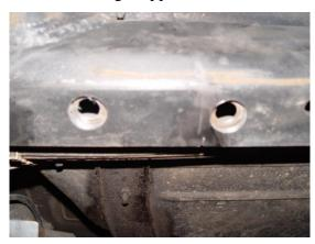
**CAUTION:** Do not over weld the bungs and distort the threads. We suggest installing a ½" bolt into the bung to protect the threads from weld splatter.
