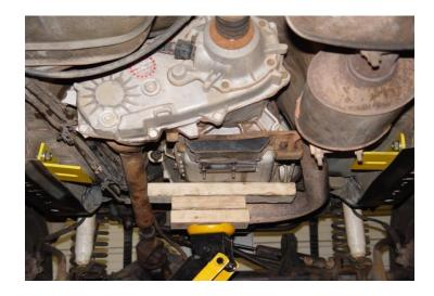
Begin the final installation of the XD Belly Pan by selecting the 6 - M10-1.5 X 30mm bolts and corresponding flat washers. Position and support the XD Belly Pan under your Jeep with the transfer case skid support against the Driver's side uni-rail.
