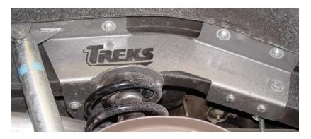
Once all holes have been drilled, locate the driver's side inner brace that was included in the kit and line it up inside the cargo area with the previously drilled  $\frac{1}{2}$ " holes. Reinstall bump stop bolts and swaybar mount bolts into bracket. Inserting the bolts from the bottom side; install upper coil mount in place using  $5 - \frac{1}{2}$ " X 1  $\frac{1}{4}$ " bolts,  $10 - \frac{1}{2}$ " washers, and 5 - nylock nuts.
