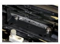
3. Install your new Diode Dynamics brackets using the provided M8 hardware in the newly uncovered holes shown in the image to the left.
