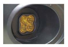
5. Using the OEM hardware, loosely install the bracket and pod in the fog pocket. Install the nuts hand-tight and do not snap the push rivets down as the pod will need to be removed to lock-in final aiming.
