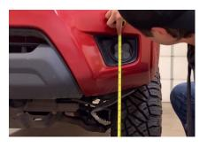
9. On your vehicle, measure the distance between the ground and the center of your SS3 pod. This is your mounting height.
