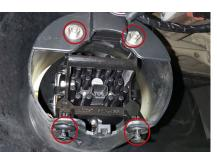
4. Unplug the fog lamp connector. Use a plastic trim removal tool to remove the two plastic push rivets along the bottom of the lamp. Holding the front face of the lamp, use a 10mm socket to remove the two nuts and gently pull the lamp out the front of the bumper opening.
