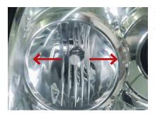
3. Check to make sure the bulb is aligned so that light is shining out to the sides horizontally. Adjust rotation if necessary.
