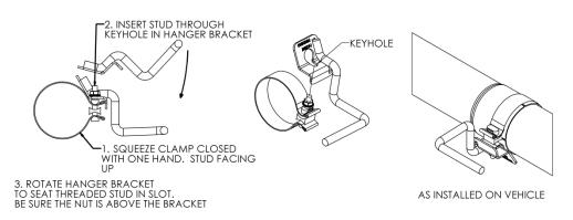
5. Place the previously assembled Hang Tight<sup>TM</sup> Hanger onto the end of the over axle pipe, leaving the clamp loose. Install the **Hang Tight<sup>™</sup>** Hanger into the factory rubber isolators. **Refer to Figure 6**
