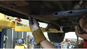
Additionally, the wings on the transmission crossmember will need to be cut in order for the part to slip on.
