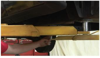
If you are keeping the body mount and the bracket on the inside on the driver side, you will have to remove and retain for reinstallation later. Alternatively, you can cut these perforated flanges off to go around them. Keep the perforated sections if you plan on replacing the body mount and bracket.
