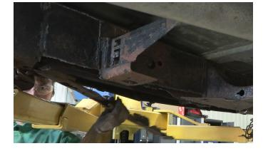
While cutting the crossmember wings, ensure you leave enough material to weld back onto the frame section.
