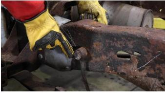
Hold the part up to the frame using the frame holes for alignment and take note of its coverage. Mark off any sections you wish to cut off, while leaving enough to weld back on to. (OPTIONAL): Coat the part with a weld-able primer or other rust inhibitor prior to installation to help prevent or reduce the risk of rust formation.
