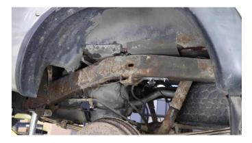
Place a set of stiffeners into place using the bolt holes and body mount brackets as reference points, and take note of any obstructions.
