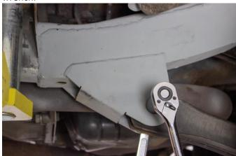
Reinstall upper control arm using 17mm socket.
