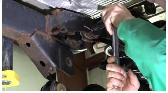
Rotate control arms down and out of the way. This may require you to loosen the axle side bolts.
