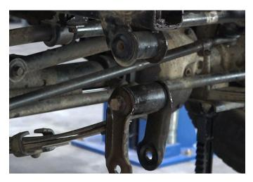
Using two 19mm sockets, remove the upper leaf spring shackle bolt and loosen the lower bolt enough to rotate the shackle down and away from the mount section.
