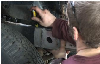
Take note of the location of the OEM sway bar bracket and mark it onto the Rust Buster part. Measure 2.375" inches from the inside edge of the rightmost hole and draw a line. The inside of the left flange will rest flush on this line.
