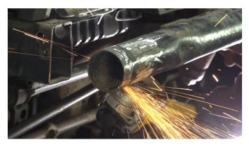
Cut away the section just inside the markings, while avoiding damage to the sway bar bracket. This will
