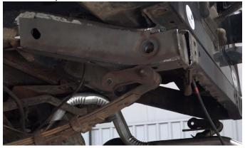
The part may fit snugly and require force. Ensure the bushing hole is visually aligned with the right
