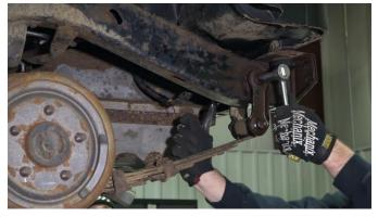
Loosen the lower bolt enough to rotate the shackle down and out of the way, exposing the frame.
