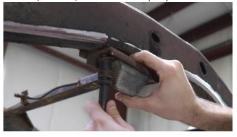
Place a set of stiffeners into place using the bolt holes as reference points, and take note of any obstructions.
