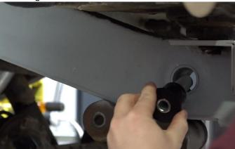
Rotate the shackle into place, send the bolt through, and secure the nut onto it. Reinstall your gas tank, cords, and tubes.
