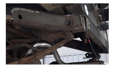
The part may fit snugly and require force. Ensure the bushing hole is visually aligned with the right side of the frame.
