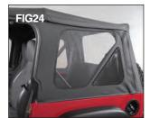
Zip down the rear quarter window zipper all the way down to the bottom of the rear quarter window. See FIGs 23 & 24.
