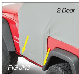
Repeat this procedure on the other side of the vehicle. Once all straps are secure, tighten each strap to secure the cover on the vehicle. (See Figs JK1, JK2 & JK3)
