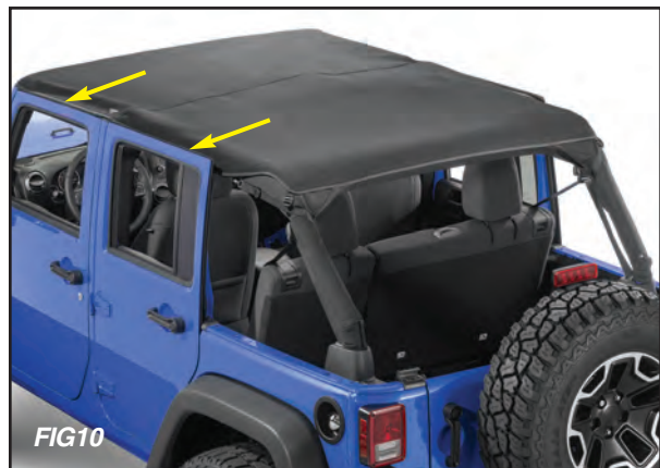
Without Factory Style Door Surrounds Bimini Plus Fabric lays inside the doors of the vehicle.
