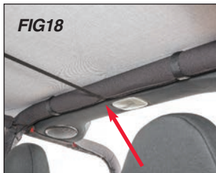
Bimini with Sound Bar: Thread center strap between sport bar hoop and soundbar.
