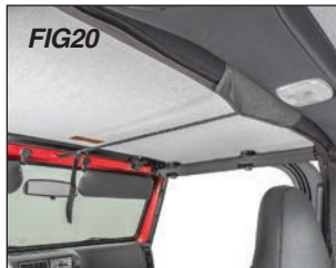
Bimini Plus with Sound Bar: Thread the center strap between sport bar hoop and soundbar.
