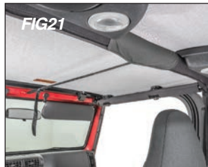
Bimini Plus without Sound Bar: Simply wrap center strap around sport bar hoop.
