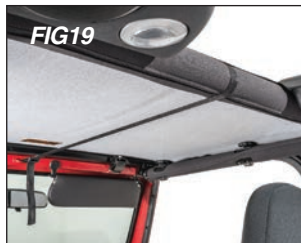
Bimini without Sound Bar: Simply wrap center strap around sport bar hoop.
