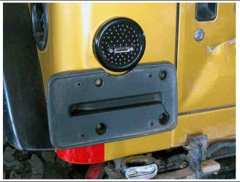
Image 13 - Example of License Plate trimming if OEM plate bracket is reused
