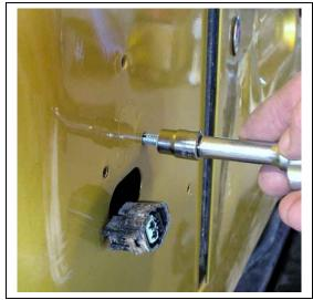
Image 7 - Threading body with self tapping screw
