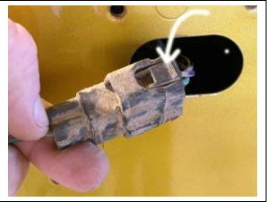
Image 3 - Press this tab to release connector
