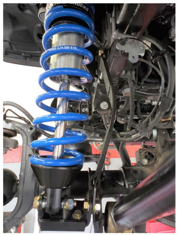
4. On axle side. Using supplied ½" bolt, washer and nut install lower end of limit strap loop to the inner factory JL shock mount tab.
