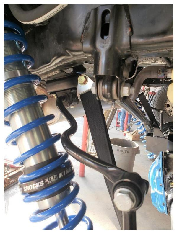
7. On rear axle. Drill/enlarge existing hole in rear lower control arm brackets to ½". Using supplied ½" bolt, washers, nut, install lower rear limit strap loop end to drilled hole in axle bracket. Use additional washer between axle bracket and limit strap loop to space limit strap off bracket. Nut can be accessed from underside of bracket by tapping nut to wrench end and inserting upwards.
