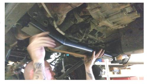
Secure the EVO HD transmission crossmember in place starting with the two bolts on each end and working your way towards the middle of the transmission crossmember.
