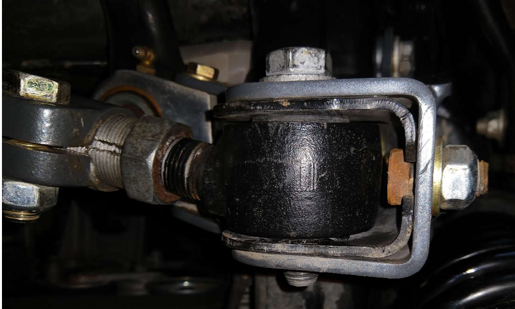
Figure 5. Synergy Mfg Track Bar Installed at the Frame
