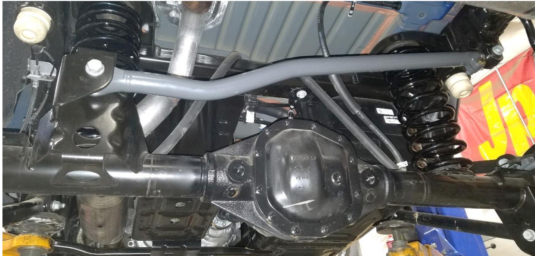
Figure 6. Correctly Installed Synergy Mfg Rear Track Bar
