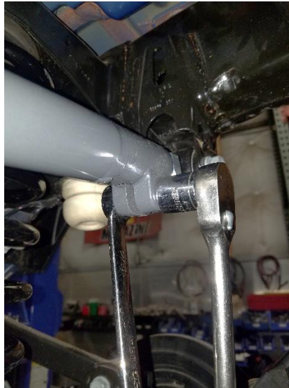
Figure 8. Tightening the Pinch Bolt and Nut
