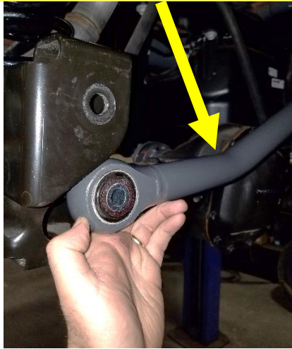
Figure 5. Installing the Synergy Mfg Track Bar at the Axle
