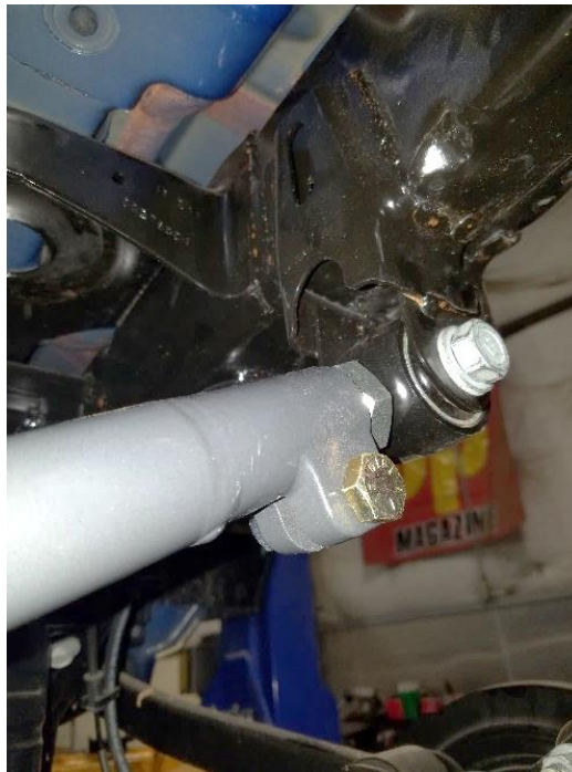
Figure 4. Installing the Synergy Mfg Track Bar at the Frame
