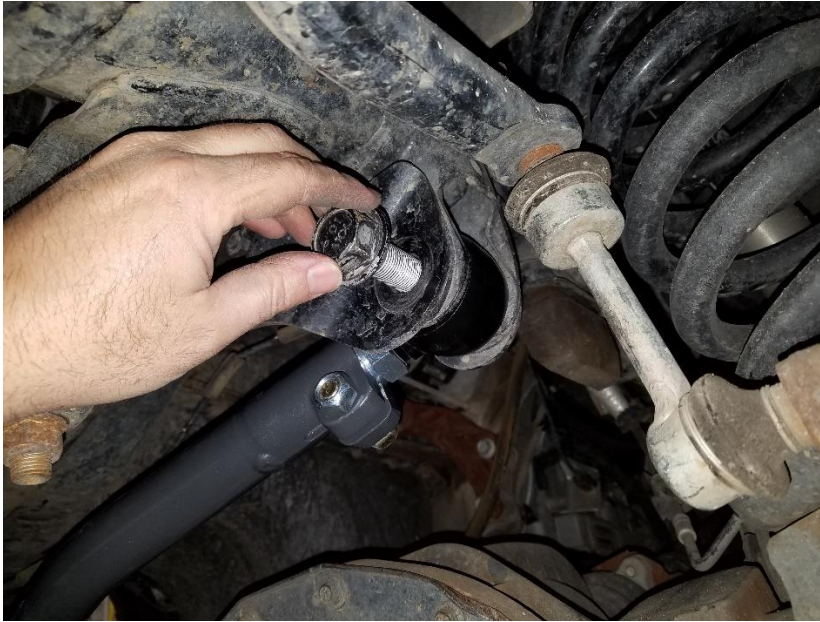
Figure 6. Installing the Frame Side Bolt
