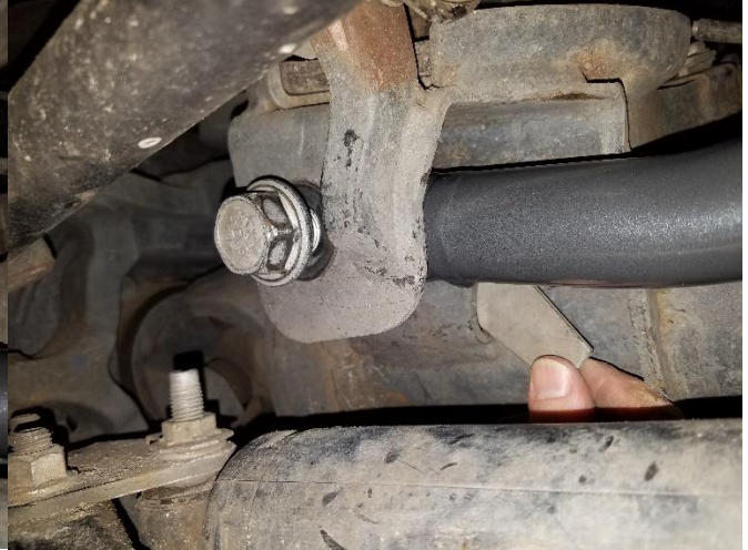
Figure 5. Holding the Flag Nut for Assembly
