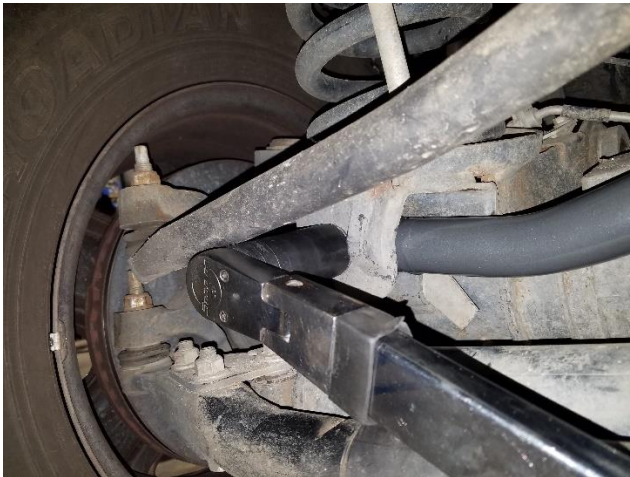
Figure 8. Torqueing Axle Side Bolt
