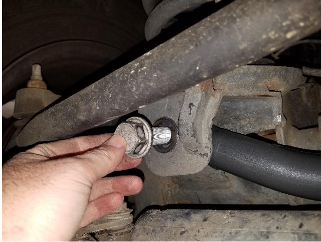
Figure 4. Installing the Axle End Bolt
