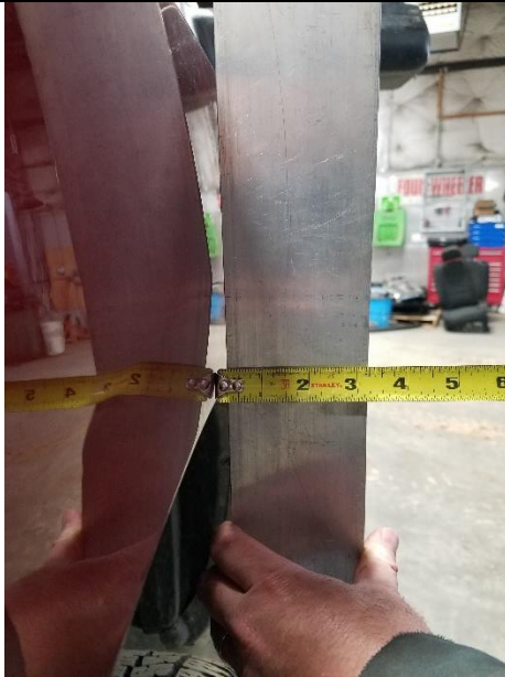
Figure 10. Measuring Axle Side to Side
