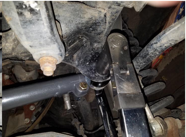
Figure 9. Torqueing Frame Side Bolt
