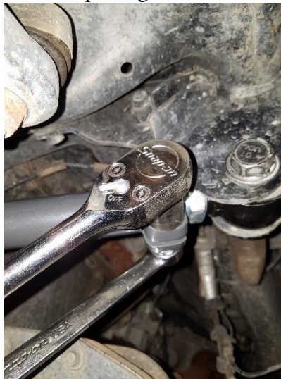
Figure 12. Tightening Pinch Bolt.
