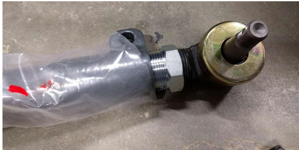
Figure 3. Double Adjuster Side of Tie Rod
