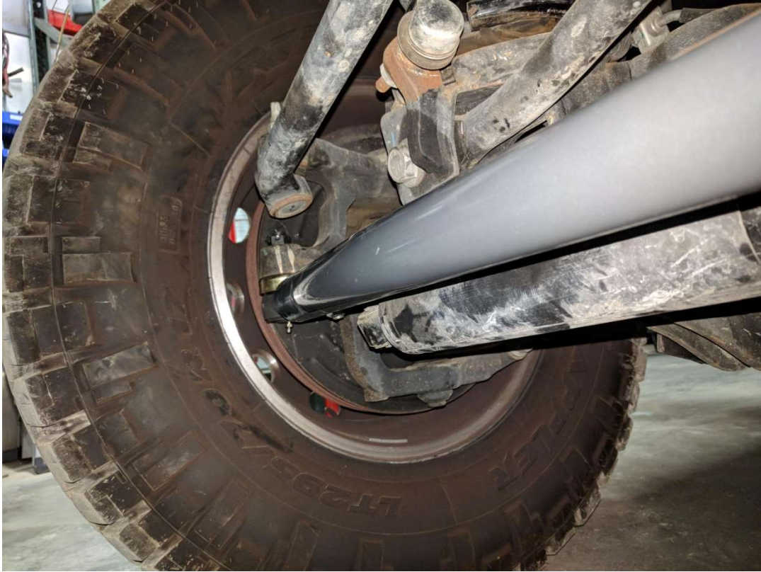
Figure 9. Tie Rod Aligned with Bend Forward and Pinch Bolts Back
