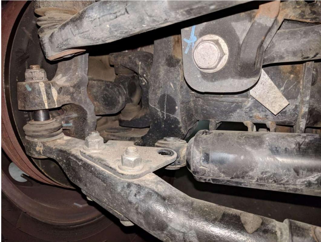
Figure 1. Steering Stabilizer Removed From Stock Tie Rod
