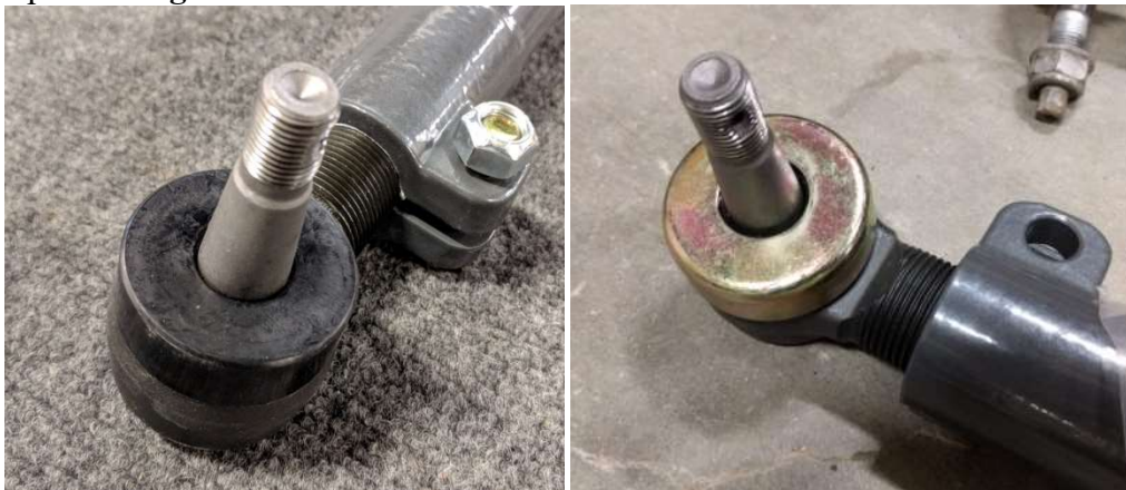
Figures 5 and 6. Dust Boots With Rubber and Metal Caps Installed
