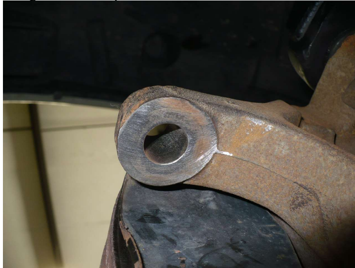
Figure 7. Steering Knuckle Arm Sanded Flat
