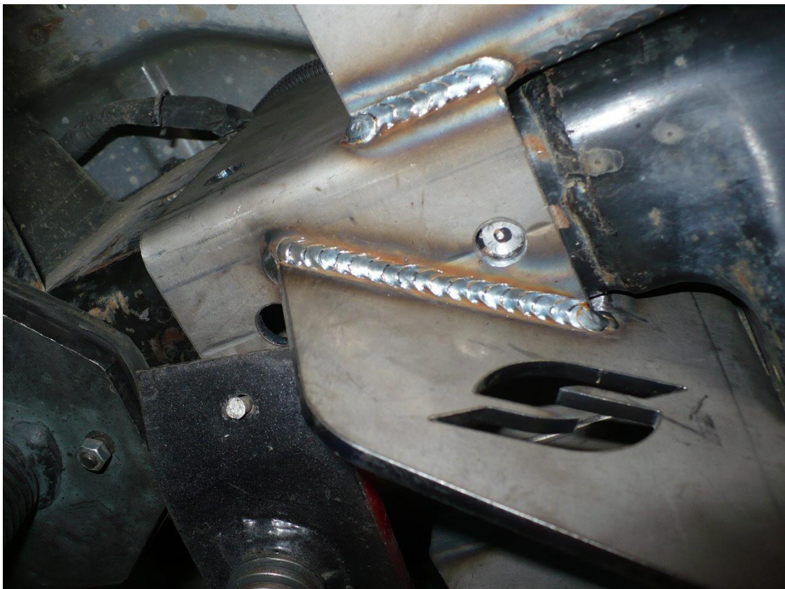
Bottom hole on frame bracket, note forward hole lines up with slot in frame.
