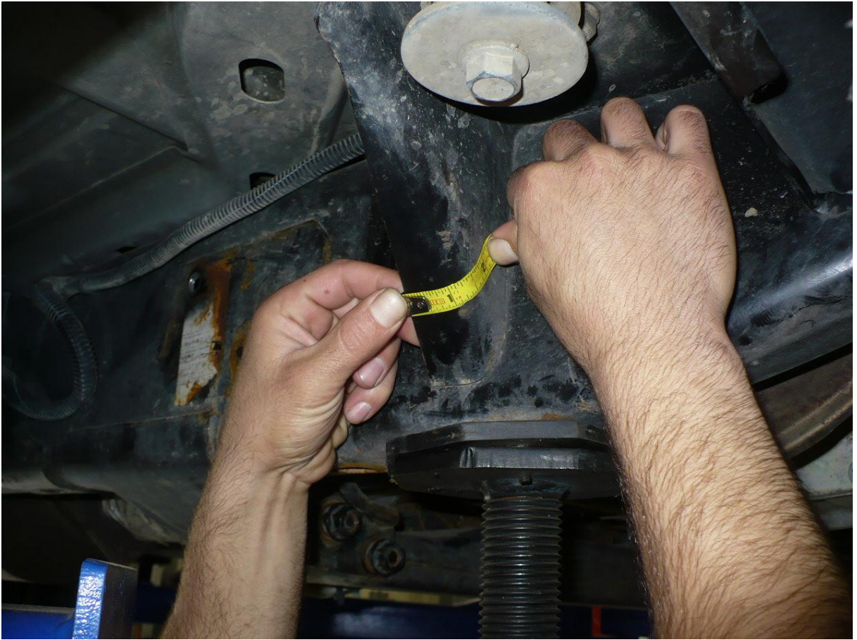
11) Trimmed drivers side body mount should appear as shown below.
