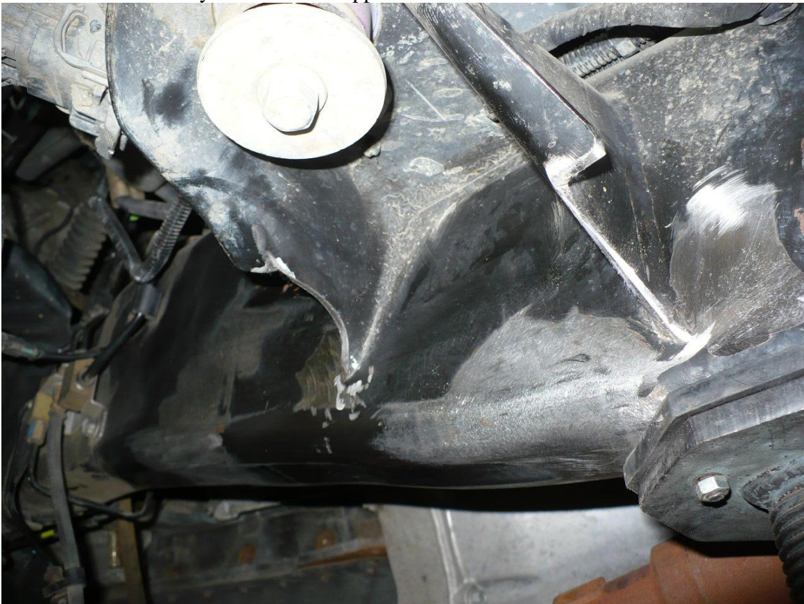
11) Trimmed drivers side body mount should appear as shown below.
