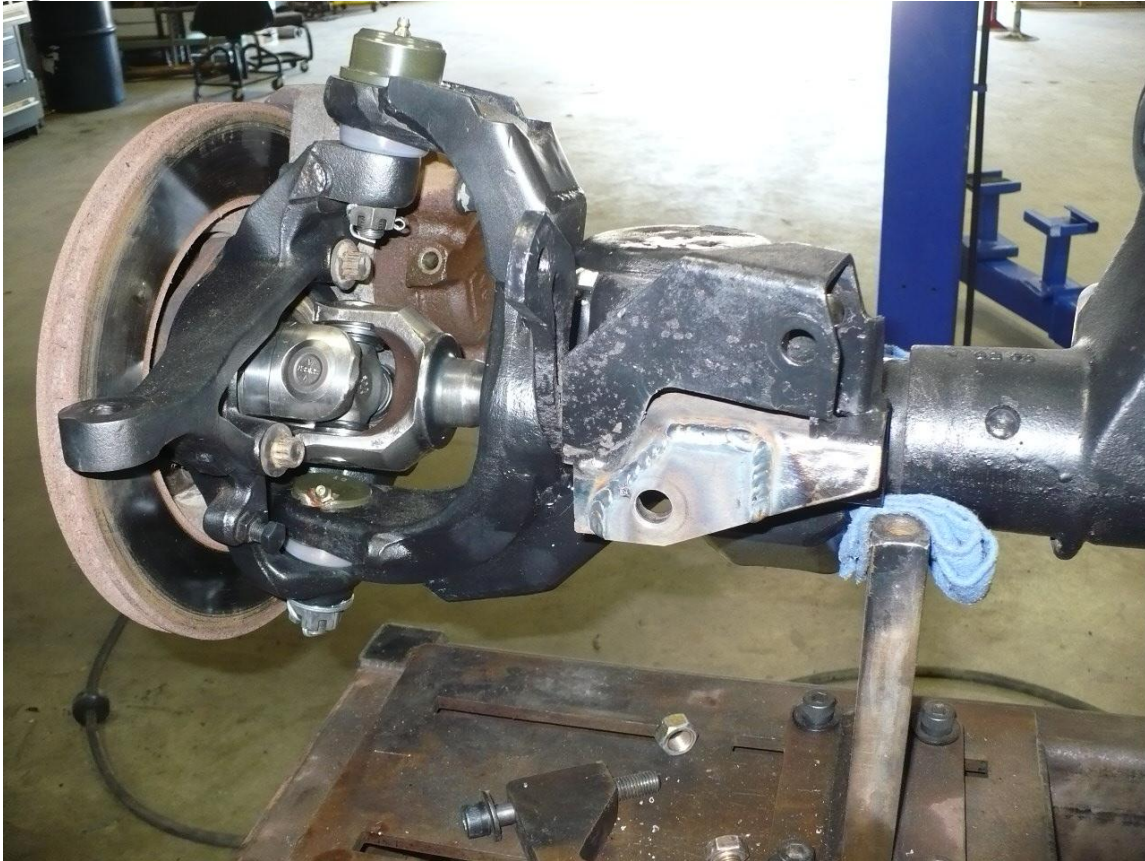
Figure 1. Axle Side Track Bar Mount Gusset Installed
