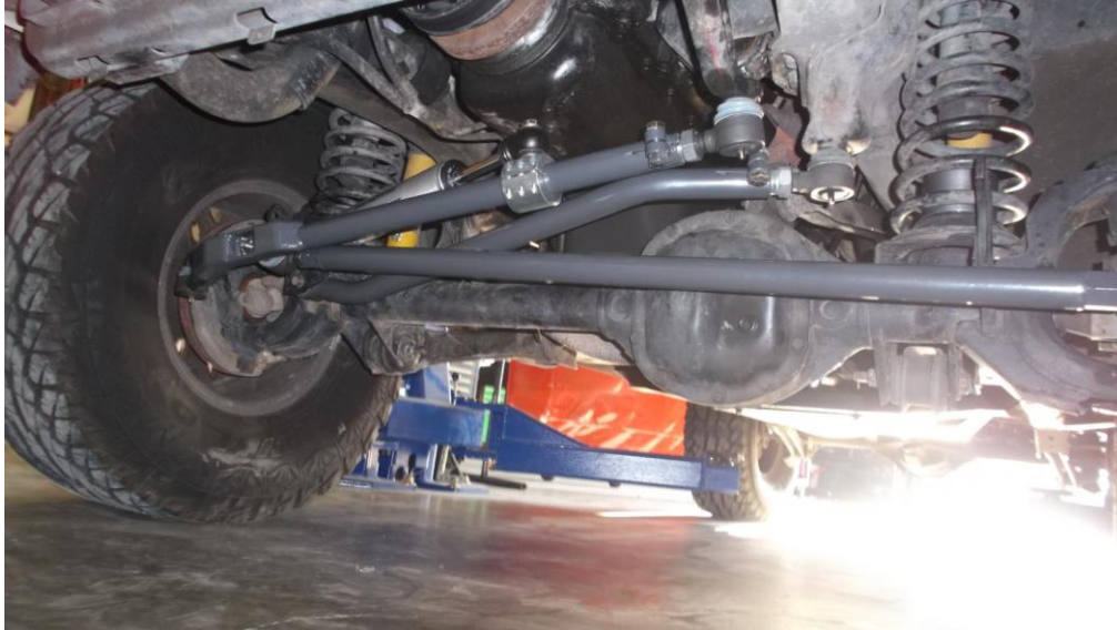
Figure 2. Installed Track Bar
