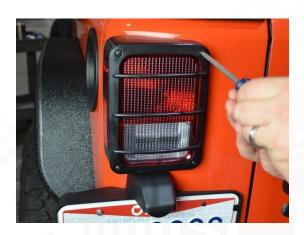
your tail light. Install two No. 10 screws and two spacers into the outside holes.
