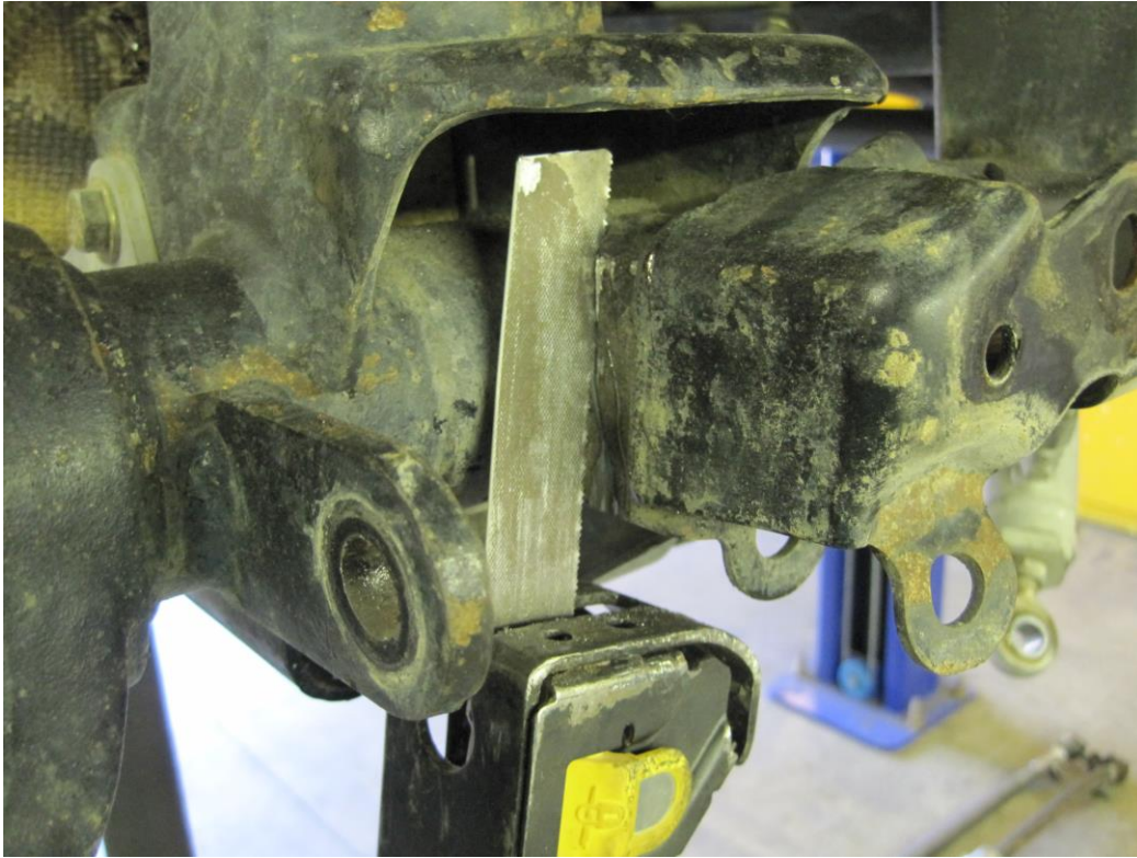
d) Remove the track bar bracket and grind smooth
