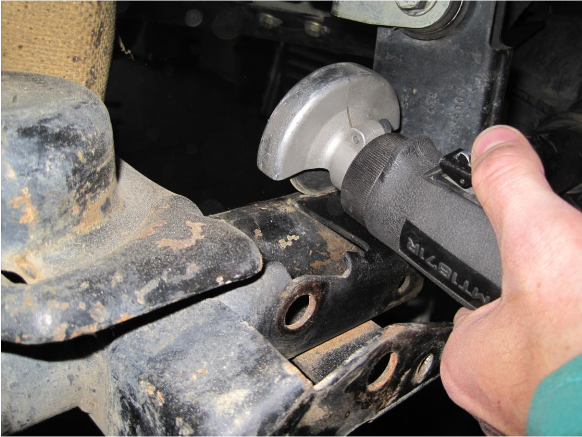
b) Cut the bottom welds with a cut off wheel
