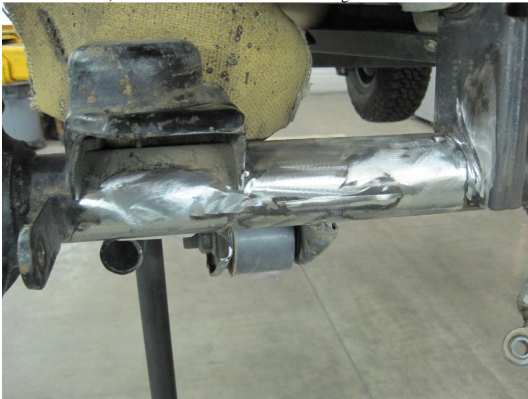
d) Remove the track bar bracket and grind smooth
