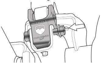
Reuse the factory hardware to mount the shock into the extension. Torque the bolts starting from the bottom to the top.
