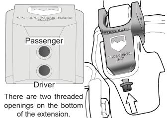
Insert the supplied M12 bolt through the middle opening followed by a washer and M12 nut. Hand tighten.
