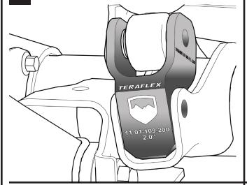
Align the extension in the axle mount and insert the supplied M8 bolt. Hand tighten.
