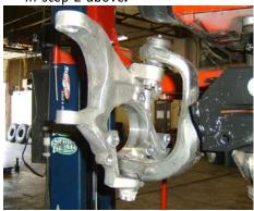
11. Install the drag link from knuckle to pitman arm. Refer to the attached drawing and be sure to use a 9/16 flat washer under the castle nut.
