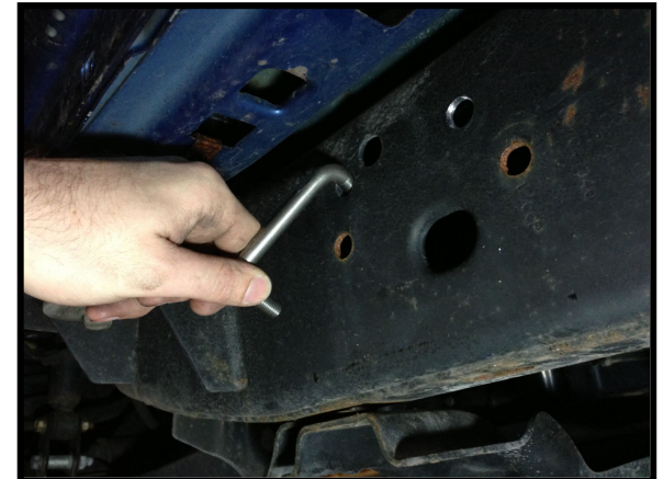
Figure 2, U-Bolt Shown without Rock Slider For Clarity. Install with Rock Slider In Place
