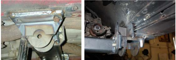
10. Grind away paint behind this bracket to prepare frame for the 3 link brace. Below are 3 pictures of how the 3 link brace connects to the 3 link mount. Do NOT use this 3 link kit without the 3 link brace!
