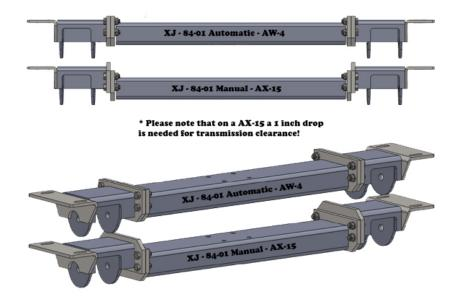
8. Center the new cross member and secure it using the two mounting holes on each side.
