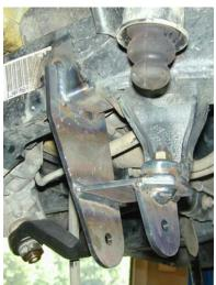
9. Adjust Johnny Joint so that the supplied 9/16s bolt easily slides through the new trackbar drop bracket.
