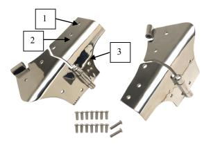
Note: The factory bolts have been installed using a thread locking cement, and sometimes are difficult to remove unless heat is applied to the head of the bolts. The factory has also put a threaded back-up steel plate inside the windshield to accept the bolts, this plate could fall inside the windshield. Loosen all the upper bolts one at a time then remove the bolts following the instructions below.
